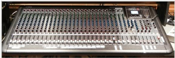
Near the bottom of the fader for each of the 32 channels, there are 3 **ASSIGN** buttons. For normal use, all three buttons should be pressed down except for the 1-2 buttons for the over the audience mics OHL & OHR, and the Ceiling Front of Stage Mics FSL, FSC, FSR. The assignment buttons send the output of each line as follows:
